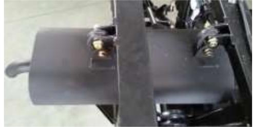
Use the following procedure to periodically purge accumulated carbon from the exhaust pipe.
