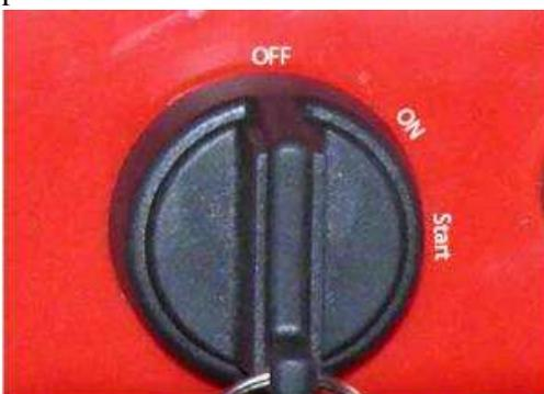
**ON:** All electrical circuits are supplied with power, the ignition system and fuel system, the headlights and taillights come on when the light switch is on.
