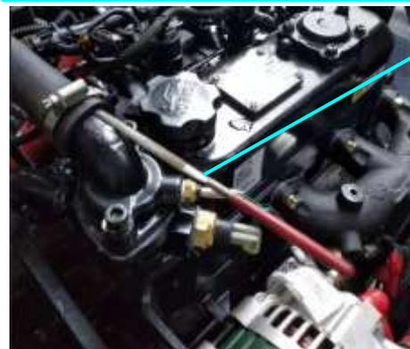
**CAUTION!** Escaping steam can cause burns. Never remove the pressure cap or plug while the engine is warm or hot. Always allow the engine to cool before removing the pressure cap or air release plug.
