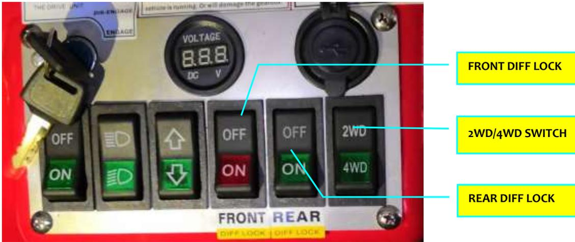
This vehicle is equipped with an electrically controlled drive mode selection. Select the appropriate drive mode according to the terrain conditions.
